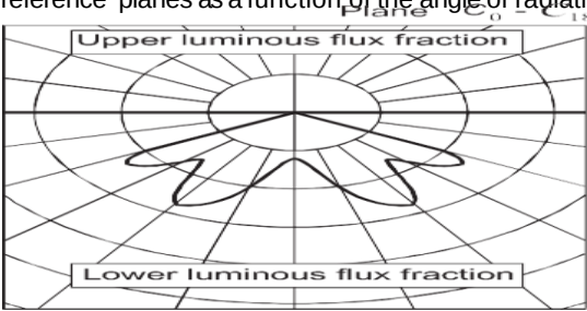
Figure I4.1: Luminous intensity distribution
